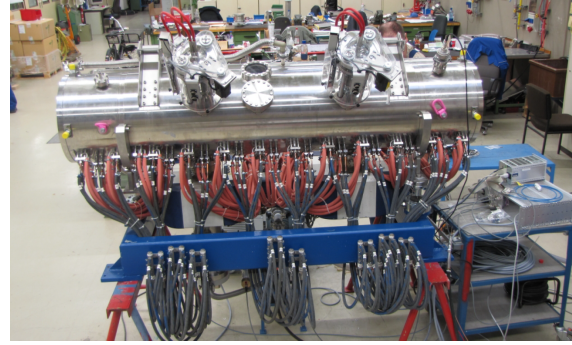
Figure 3.2: HLI-RFQ tank during assembly at GSI [78].
