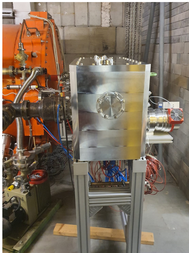
Figure 4.43: Prototype tank in the RF test bunker at GSI 10 .
