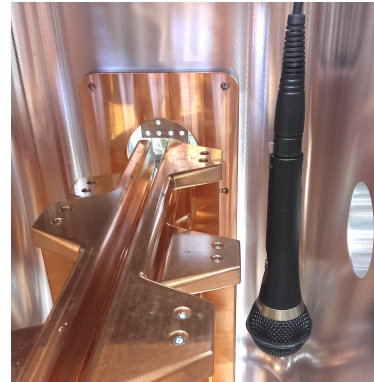
Figure 4.29: Microphone suspended in the prototype tank.
