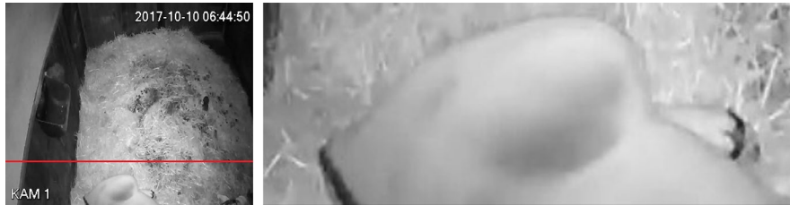
FIGURE A1 Example of an event of high truncation. The image is likely to be misclassified as standing without postprocessing. The l.h.s. shows the recorded image and on the r.h.s. the result of the object detection phase is shown
