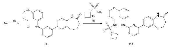
**Scheme 2.** Preparation of sulfamoylaminoalkoxy-substituted compounds **14a–g** exemplified by the synthesis of **14d**. Reagents and conditions: (i) 1-bromo-3-chloropropane, Cs<sub>2</sub>CO<sub>3</sub>, ACN, reflux, 2 h, 25% and (ii) K<sub>2</sub>CO<sub>3</sub>, NaI, DMF, 80 °C, 22 h, 34%.
