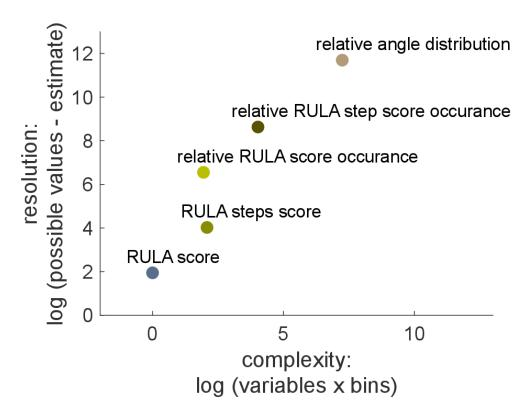
**Figure 4.** Complexity versus resolution. The complexity was based on the number of variables used in the individual steps. The resolution is based on the number of scores or on the number angles, where  $1^{\circ}$  bins were used.
