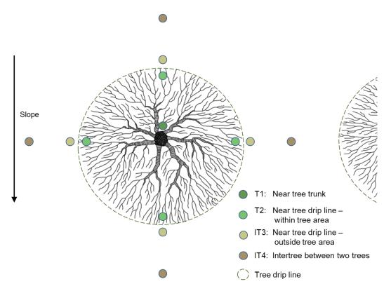
145 Figure 4: Schematic diagram of soil sampling locations in the tree and intertree area.
