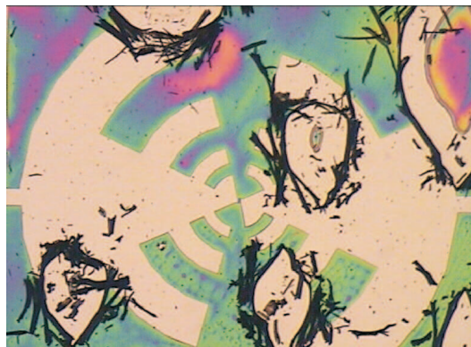
Figure 3.17.: Oxidation (black islands) of LTG-GaAs photomixers with Bragg reflectors exposed to air.
