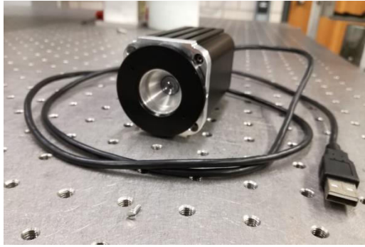
Fig. 4.4. Camera enclosure with a lens holder and USB connection.
