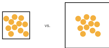
Figure 5.15: Illustration of cell-size overestimation. Black square displays the grid cell and yellow dots the particles inside the cell.
