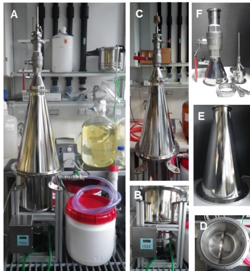
Fig. S2: Replica of the Munich Plastic Sediment Separator (MPSS) originally published by Imhof et al. (2012). Overview of the MPSS (A), sediment chamber (B), dividing chamber and filtration unit attached to the standpipe (C), interior of the sediment chamber (D), standpipe (E), dividing chamber (left) and filtration unit (right) which are connected by a bayonet joint (front, F).
