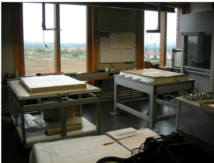
Figure B.1: The table for the frame assembly (right) and the vacuum table for the gluing of the back panel (left). The aluminum plates are especially designed and machined with very high precision of a maximum deviation of less than 0.1 mm.
