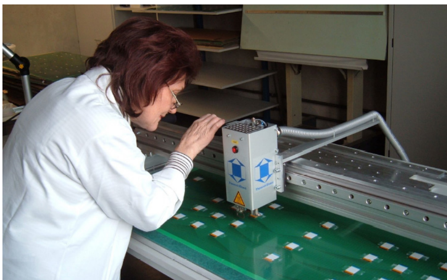
Figure B.4: The solder machine used for soldering the flat ribbon cables to the PCB. The correct position of the soldering iron with respect to the cables is ensured by latches.
