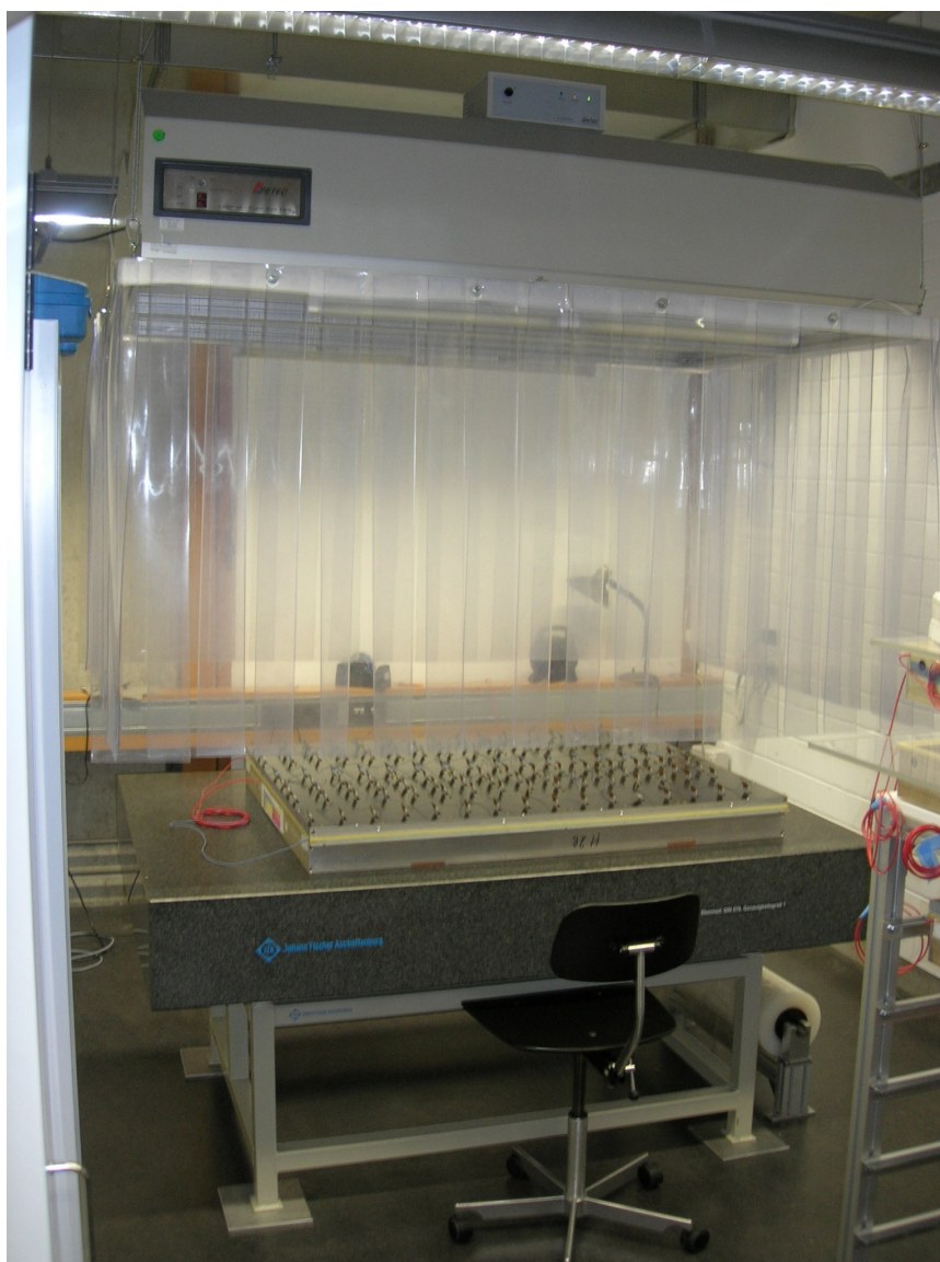
Figure B.2: The extreme precise and vibration-less stone table. The laminar flow box on top of it provides an almost dust free air flow. The table is used for the final assembly of the chambers and, due to the small vibrations, for repairs.
