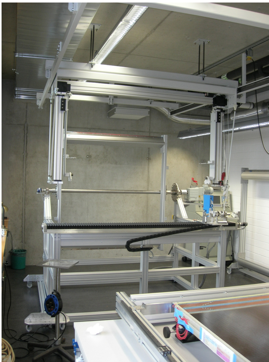
Figure B.3: The winding machine with the wire tension meter (blue) and a large aluminum frame. On the ceiling a special lifting device for the heavy aluminum frames ( \sim 100 kg) was mounted.
