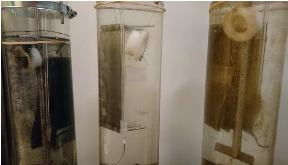
Figure SI-1. Photograph of three sediment cores. Left core is a resuspended PAC treatment, middle core is not resuspended, and the right core is resuspended without PAC. Note the black color of PAC on the walls and passive samplers to the left, the translucent SPMD in the static condition in the middle core, and the brown color of sediment or clay on the walls and passive samplers to the right.
