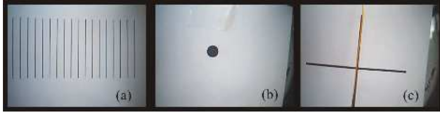
Figure A.9: Photographs from the camera used for image calibration (a) for x - y pixel calibration, every line is 5\text{ mm} apart in shown picture (b) to determine the centre and (c) to determine the tilt of the camera.
