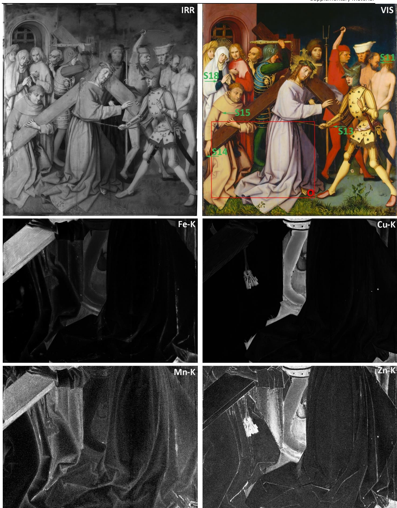
Suppl. 5 H. Holbein the Elder, “Bearing of the Cross” (Inv. No. HM 15), inside of the outer wings, High Altarpiece of the Dominican Church. Top row, left to right: Conventional IRR image (900–1700 nm) and visible light image (VIS) with mapping of MA-XRF scans performed and samples S12–S15 and S18. Bottom rows: MA-XRF elemental maps of Fe-K, Cu-K, Mn-K and Zn-K.
