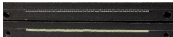
Figure 3: Interface from scintillating fibres (square, yellow, bottom) to light guiding PMMA fibres (round, clear, top).
