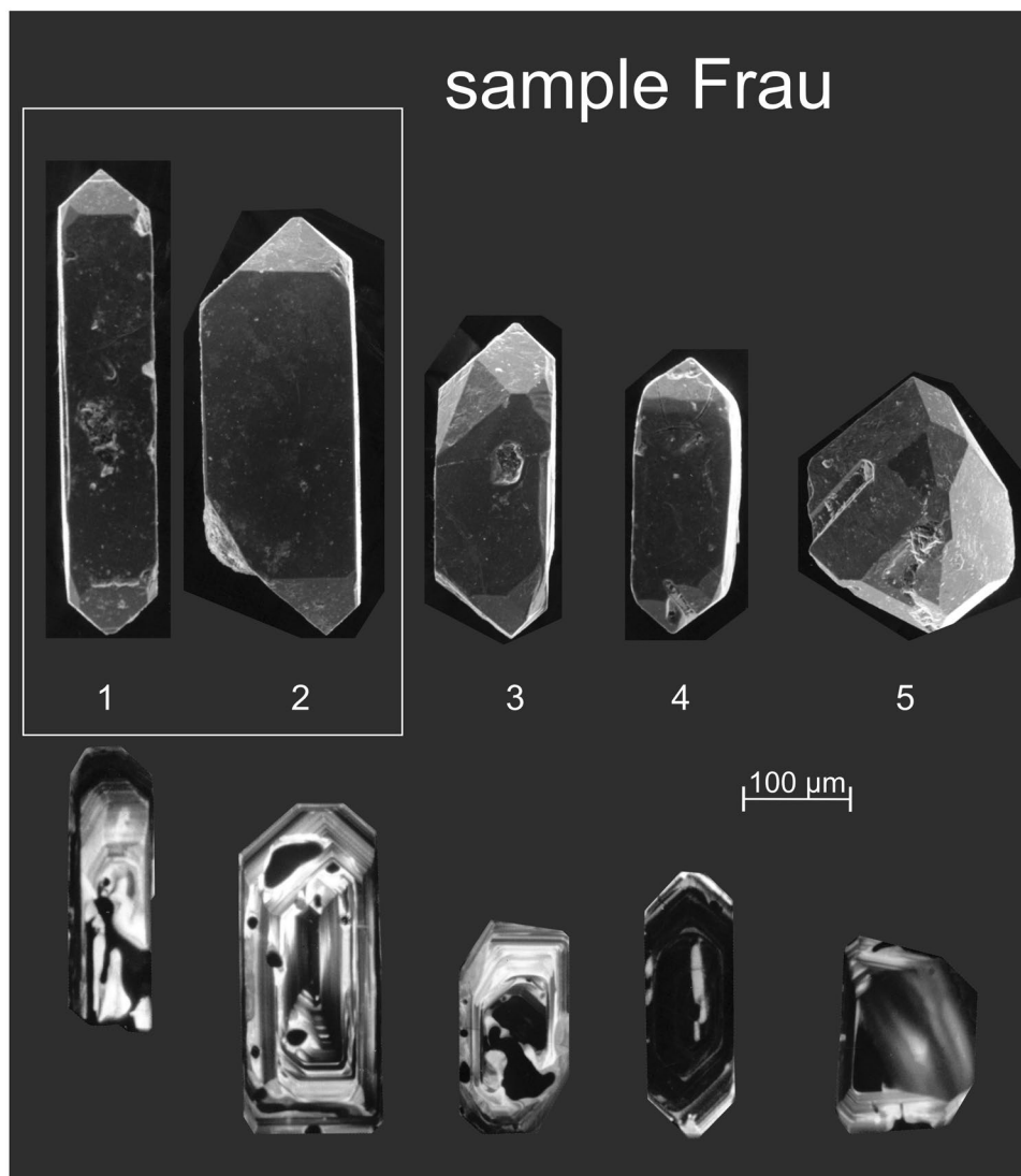
Fig. 3 Zircon SEM- (upper row) and CL-images (lower row) for selected zircon grains from sample Frau. Note that the same grains are shown in the upper and lower row. For dating with CA-ID-TIMS the most idiomorphic grains were chosen (outlined grains 1 and 2) to avoid dating of xenocrystic zircons
