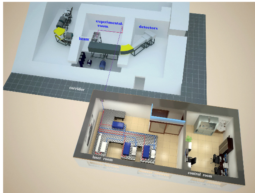
Figure 12. 3d view of the setup GaLS (Dubna) for selective laser ionization and separation of heavy transfer reaction products.
