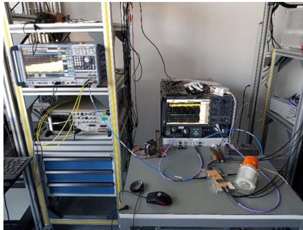
Figure 7-30: Up-converter measurement setup for output spectrum measurements.
