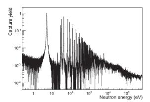
Figure 1. Capture yield obtained after normalization and background subtraction. The n\_TOF data shown here are collected with  $C_6D_6$  detection system.
