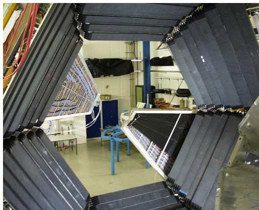
Figure 2.5: The META detectors (view from the target region). All 6 sectors of TOF are visible. Two opposite sectors are also equipped with the Pre-Shower detector. Currently all 6 sectors of the Pre-Shower detector are installed.
