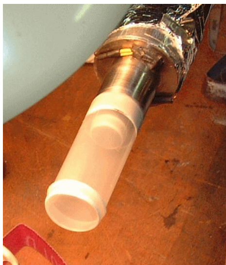
Figure 2.2: View of the liquid hydrogen target vessel. The entrance window is glued on a stainless steel cylinder with a diameter of 1.5 cm, whereas the target vessel diameter is 2.5 cm.
