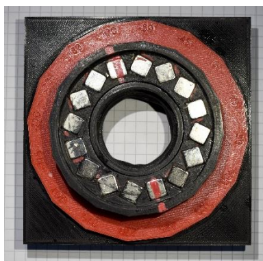
Figure S15. Image of the quadrupolar/dipolar ring-type magnet used for magnetic guidance experiments. [5]
