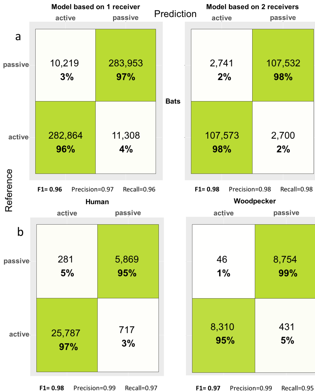
Fig. 3. (a) Confusion matrix for the one-receiver- (left) and two-receiver (right) models. (b) Confusion matrix for different activity levels simulated by humans carrying transmitters (left) and based on the observed behaviour of a middle spotted woodpecker (right).
