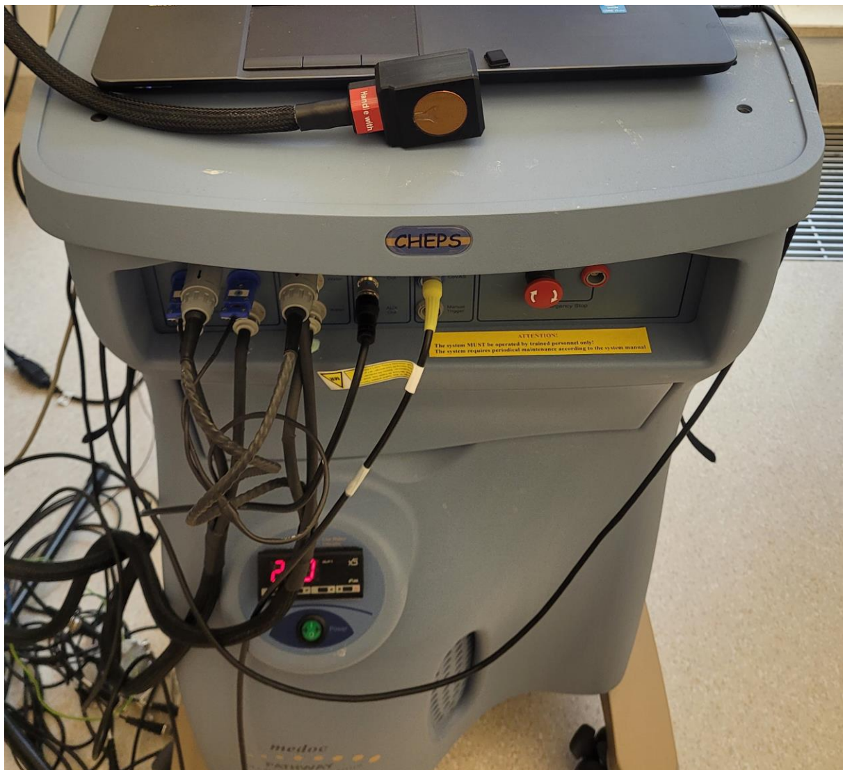
Figure 4: the thermal stimulation device MEDOC PATHWAY Pain and Sensory Evaluation System (Medoc Limited, Ramat Yishai, Israel), with the thermode for the stimulation with contact heat in the top-middle of the picture. The thermal probe of the stimulation device delivers short heat bursts by increasing its temperature at a fixed rate of 70°C/s and selectively activates A- and C fiber nociceptors if an adequate peak temperature is chosen.
