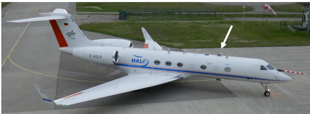
Figure 5: Photo of the HALO. The white arrow indicates the LiF-OH inlet.
