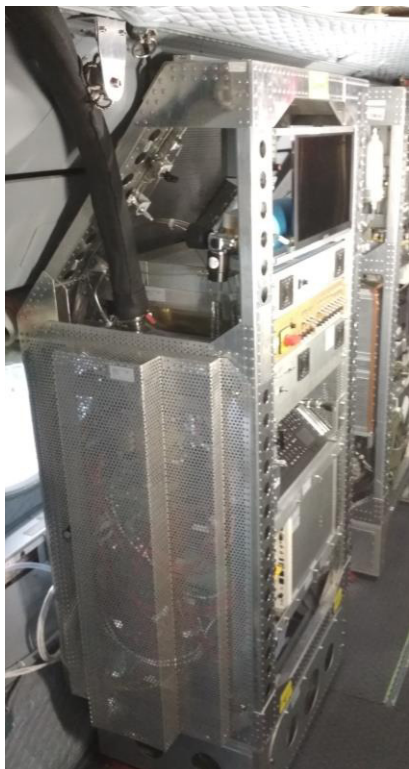
Figure 4: Photo of the SCORPION-TOF-MS installed on board the HALO. The black line in the upper left corner is the inlet line covered by thermal insulation.
