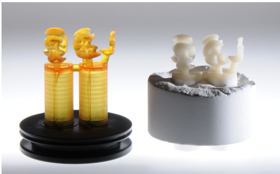
FIGURE 7 3D-printed components prepared for trixpress muffle (left); pressed restorations fixed at press sprue (right)
