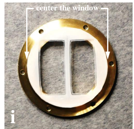
Check that window, spacer and lid are perfectly centered and the spacer is still sticking completely.
