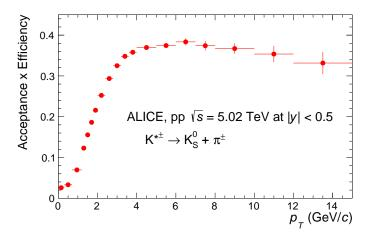
**Figure 2:** Acceptance×Efficiency as a function of  $p_T$  for  $K^{*\pm}$  mesons, detected by their decay to  $K_S^0 + \pi^{\pm}$ , with  $K_S^0$  reconstructed by their decay to  $\pi^+ + \pi^-$ . The  $K_S^0 \rightarrow \pi^+ + \pi^-$  branching ratio is included in the efficiency estimation. Statistical uncertainties are shown with error bars.
