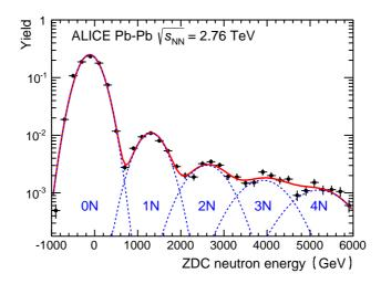
**Fig. 1:** Energy deposit in the Zero-Degree Calorimeters. The curves correspond to Gaussian fits for 0, 1, 2, 3, or 4 neutrons entering the calorimeter. The plot is for events satisfying the requirements (i)–(vi) described in the text.
