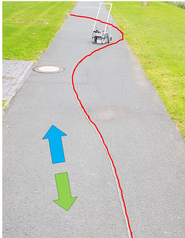
Figure 3.4: Data recording setup on the footpath asphalt application area for the teach-and-repeat scenario. First, a rope (in the image traced by the red line) is put on the ground in an arbitrarily chosen configuration. Then, we move the recording platform along the rope while recording image sequences. The aluminium profiles attached to the sides of the recording platform act as visual guidance for tracking the rope. For two sequences (green arrow, as seen in the image), we follow the rope aligning the left profile with the rope while moving in the direction of the viewer, and for two further sequences (blue arrow), we follow the rope while moving away from the viewer aligning the right profile with the rope.
