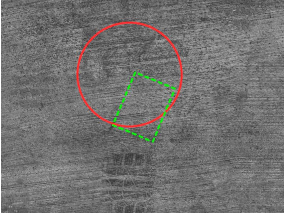
Figure 1.1: Visualization of the map-based absolute localization task, where the query image pose is estimated in respect to the reference images. Images are taken from the garage concrete dataset of our HD Ground Database [Schmid et al., 2022]. The background presents the mapped reference images as an image stitching, and the true query image pose is shown by a green dashed border around the image. Depending on the localization mode, we are either considering all reference images for potential overlap with the query image ( global map-based localization ), or an available query image pose estimate allows to consider only the reference images of a local area ( local map-based localization ). Here, we assume to have a pose estimate available according to which the query image is located in the red circle. It is useful to consider only the closest reference images to the estimated query image position for potential overlap, e. g. one could use all images with overlap to the circle area.
