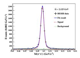
Figure 2. Fit to the  $M(\pi^+\pi^-)$  distribution at  $\sqrt{s} = 2.125$  GeV, where the black dots with error bars are data, the blue solid curve is the total fit result, the green dashed curve indicates the fitted background shape, and the red dashed curve is the fitted signal shape.
