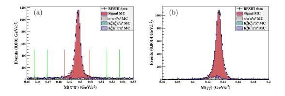
Figure 1. Distributions of (a)  $M(\pi^+\pi^-)$  and (b)  $M(\gamma\gamma)$  at  $\sqrt{s} = 2.125$  GeV, where the (black) dots with error bars are data, and the shaded histogram are stacked MC samples of signal process,  $\pi^+\pi^-\pi^0\pi^0$ ,  $K_S^0K_L^0\pi^0\pi^0$  and  $K_S^0K^{\pm}\pi^{\mp}\pi^0$ . The region between red arrows is the signal region, and the regions between the green arrows are the sideband regions.
