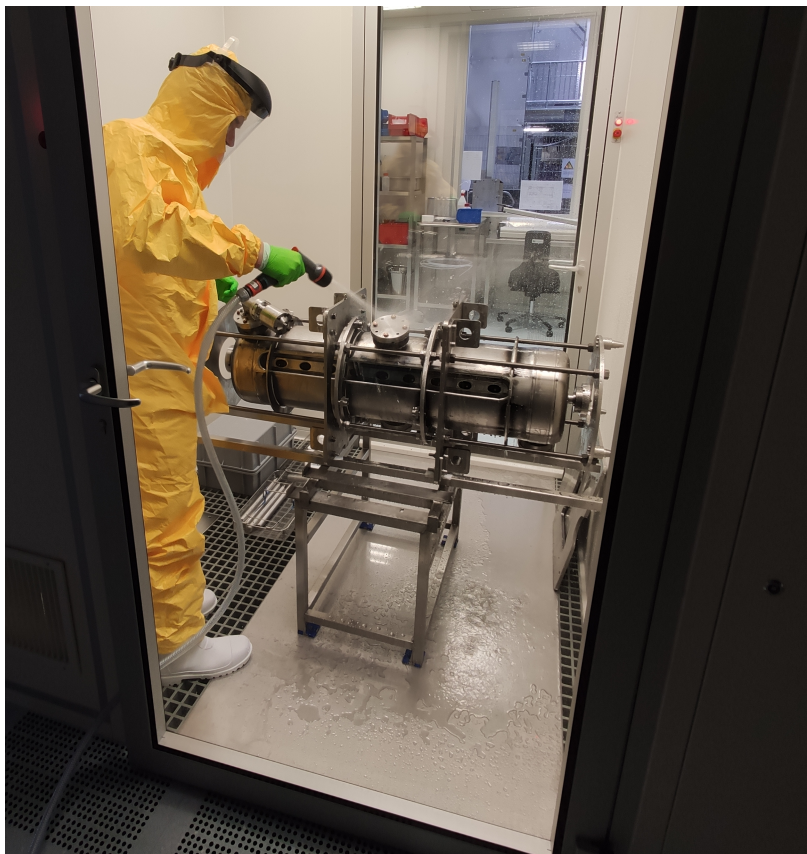
Figure 6.9: The cavity was cleaned from residual dust with ultra-pure water.
