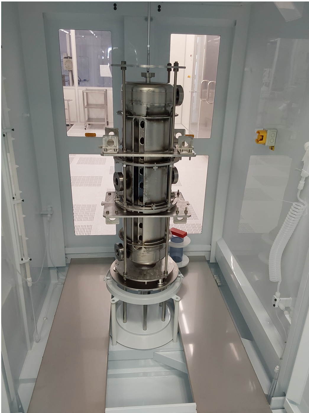
Figure 6.10: HPR setup at HIM: The cavity is positioned on an adjustable rotating table, from the top the lance is injected into the cavity through a beam axis flange.
