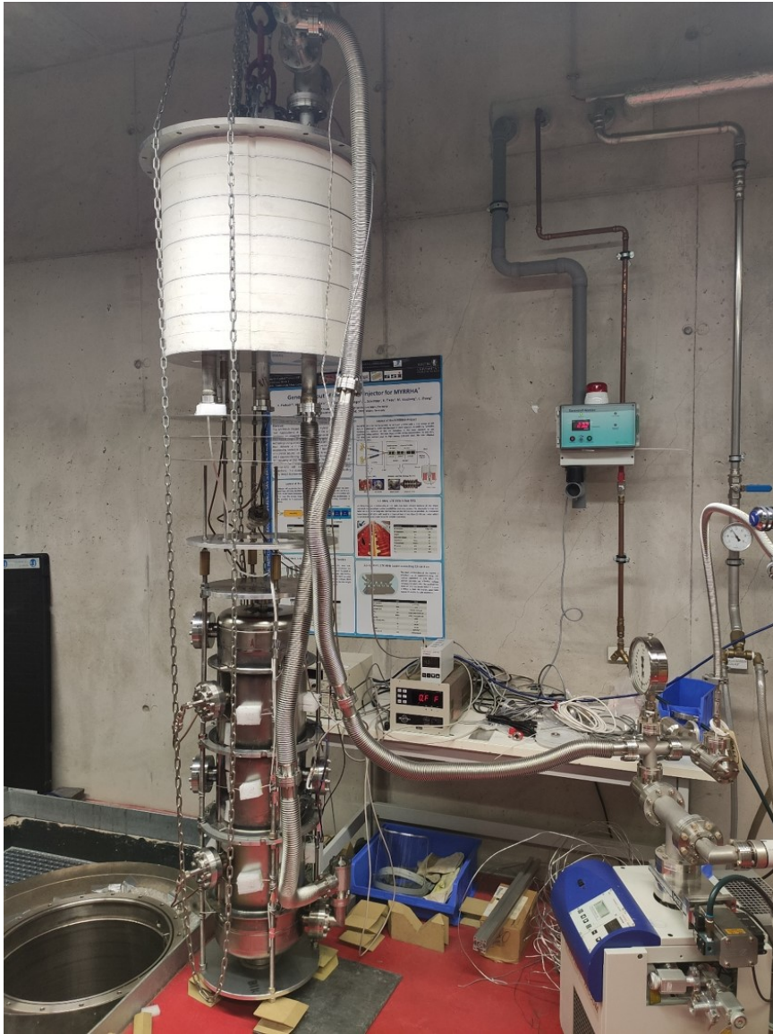
Figure 7.1: Experimental setup with the 360 MHz CH cavity before insertion into the cryotank.
