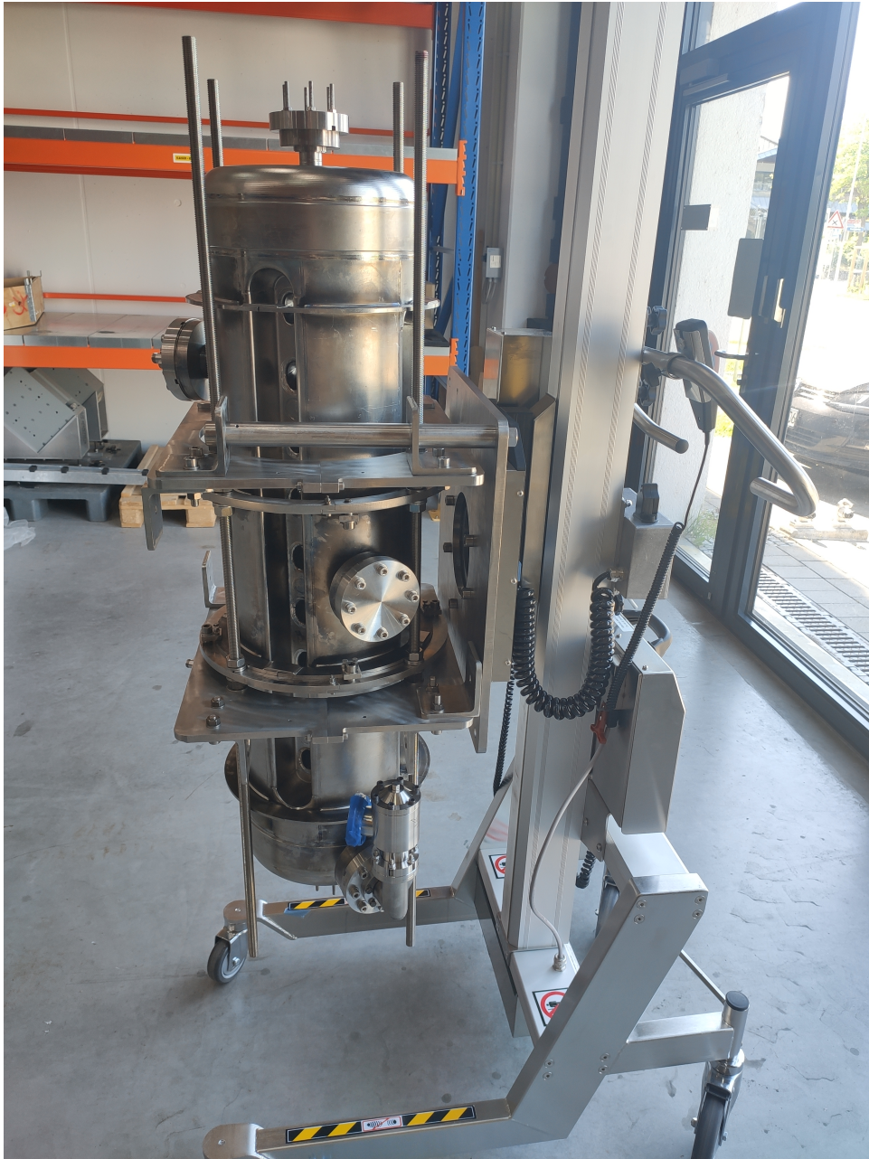
Figure 6.7: The mount was successfully tested with a mobile lifter in the experimental hall at HIM.
