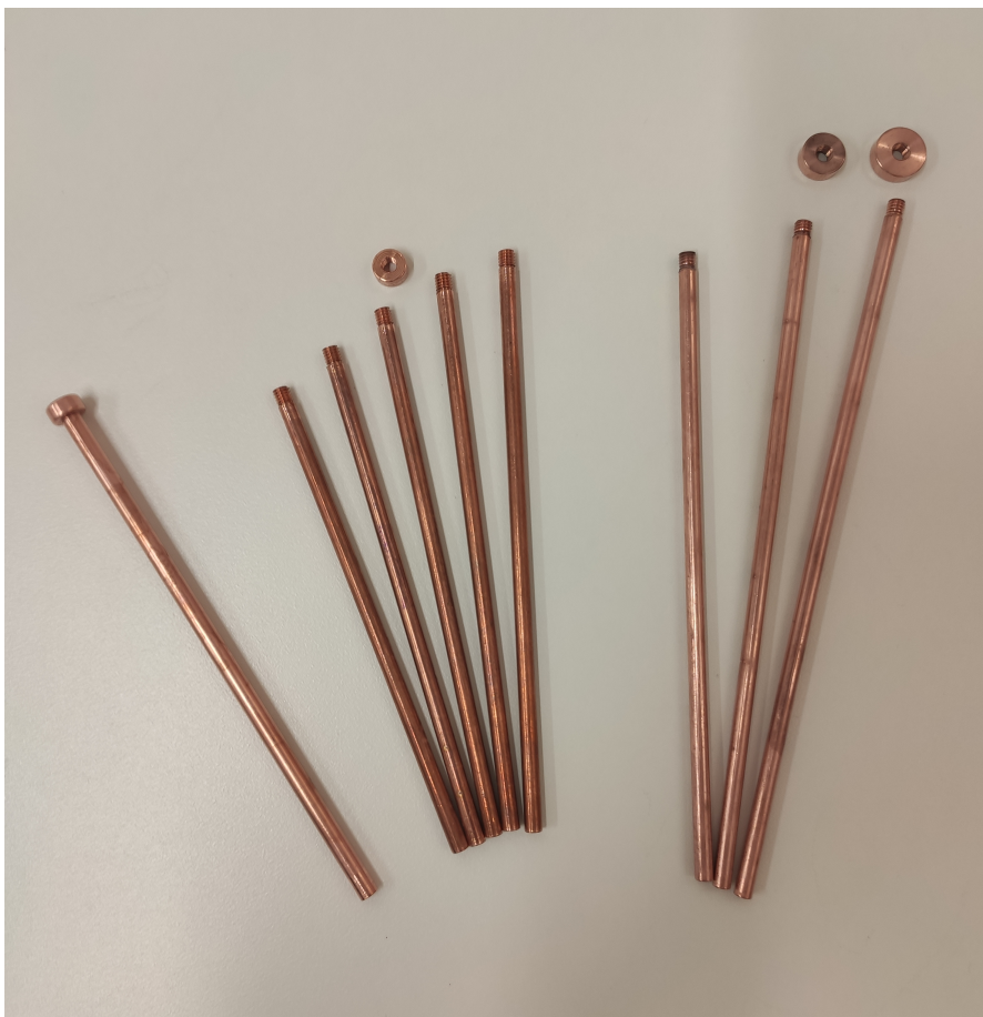
Figure 2.7: On the left side, the original heavily overcoupled coupler is shown. In the middle are the dummy couplers of decreasing length. On the right are couplers for critical coupling at room temperature.
