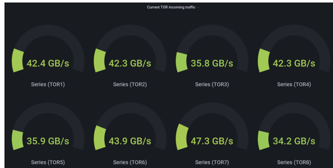
Figure 6.26: Distribution of the traffic from FLPs to EPNs across the InfiniBand ToRs during a Pb-Pb test run with 60 Hz time-frame rate and 200 EPNs (88 Hz nominal).
