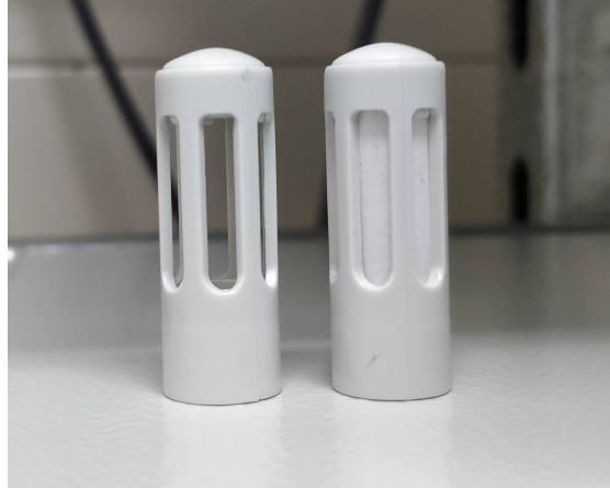
Figure 6.11: Protective caps of the temperature sensors. Left - paper inlet removed, right - original version.
