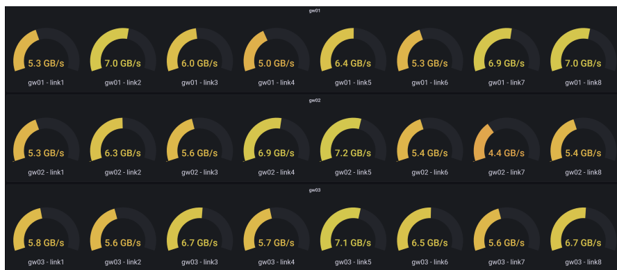
Figure 6.30: Link balancing with the new firmware 8.1.3050 with improved hashing during benchmarking.
