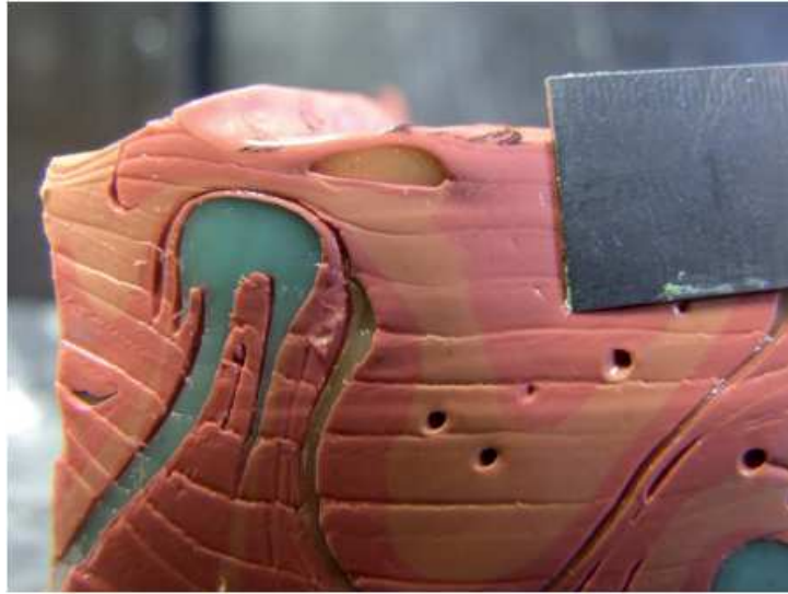
Figure V.1: Part of the experiment 1 without initial perturbations, where a diapir coming from the lower PDMS layer pierces the upper PDMS layer because this last layer is so thin, and so the rising diapir cannot use this weak plane to reach the top of the model.
