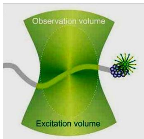
Figure 24 The schematic diagram shows the optically defined observation volume ( 250 \text{ nm}^3 ) for labelled molecule (Haustein and Schwille, 2004)
