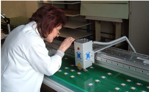
Figure 1: Soldering ribbon cables to the pad plane.
