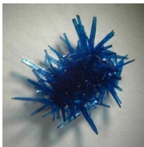
Figure 58: Crystals of the polymer [\text{Cu}(\mu\text{-ox})(\text{H}_2\text{O})(4\text{-apy})_2]_n .
