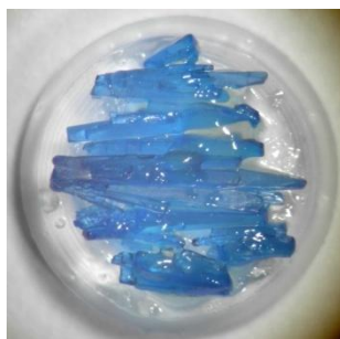
Figure 62: Sample holder with the crystals oriented in the needle direction.
