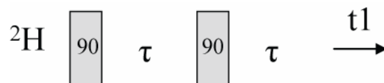
Figure 16. Schematic diagram of the quadrupole echo experiment. The quadrupole echo is used to enable static experiments with direct detection of fast relaxing quadrupole nuclei with large spectral width [191].
