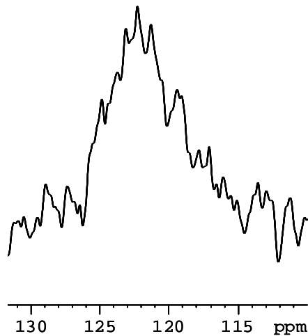
Figure 3.12: ^{15}\text{N} CPMAS NMR spectra of ^{15}\text{N} tyrosine labeled LmrA reconstituted in lipid vesicles. Spectra recorded at 8 kHz MAS spinning frequency and 253K. Approximately 250 K scans were accumulated per spectrum.
