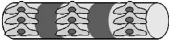
Figure 18: Schematic representation of biological surface functionalization: binding of adherent cells onto the electrode.
