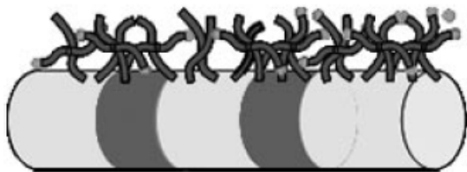
Figure 17: Schematic representation of chemical surface functionalization: binding of polymer chains onto the electrode.
