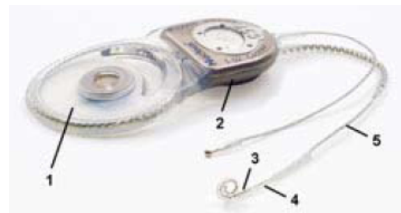
Figure 1: The implantable portion of the cochlear implant: (1) Transmitter coil in a silicone sheath; (2) Electronics enclosed in a titanium casing; (3) Electrode with platinum contacts in a silicone array; (4) Cochleostomy site; (5) Silicone cable in the middle-ear/mastoid region.
