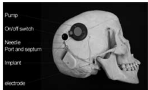
Figure 22: Schematic structure of a cochlear implant with integral micropump (MedEl GmbH) showing a septum port between the implantable pump (i.e. the circular structure on the right) and the implant (left).
