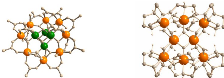
Figure 3.5: Illustrating the chemical structure of two single molecule magnets. Left panel: the \text{Mn}_{12} -acetate ( \text{Mn}_{12}\text{O}_{12}(\text{CH}_3\text{COO})_{16}(\text{H}_2\text{O})_4 ). The \text{Mn}^{4+} -ions are depicted in green, the \text{Mn}^{3+} -ions in orange. Right panel: a \text{Fe}_8 -compound ( (\text{tacn})_6\text{Fe}_8(\text{O})_2\text{OH}_{12}(\text{H}_2\text{O}) ). The \text{Fe}^{3+} -ions are represented by orange spheres.
