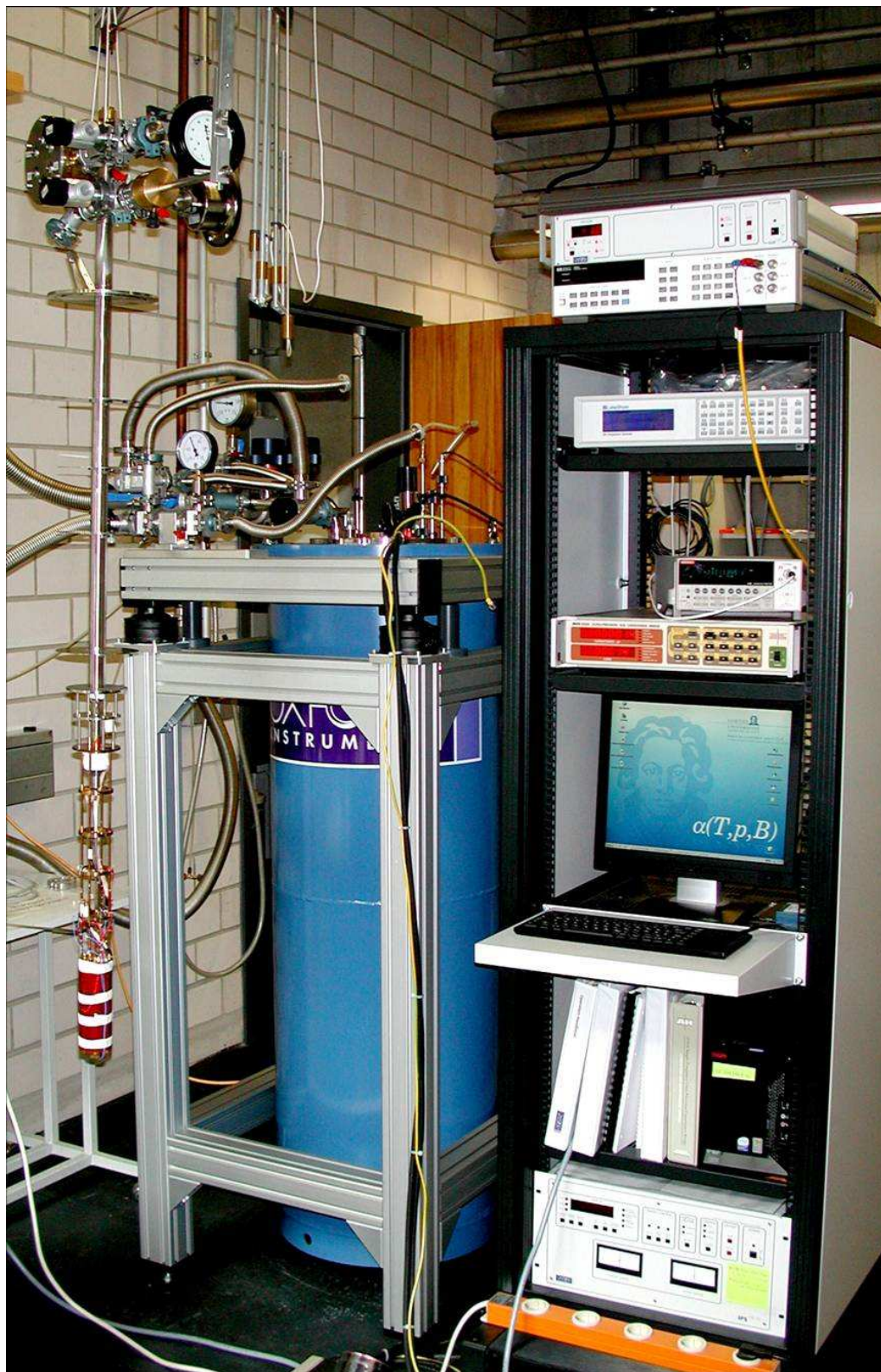
Figure 2.2.8: Picture of the whole setup ‘thermal expansion under pressure’.
