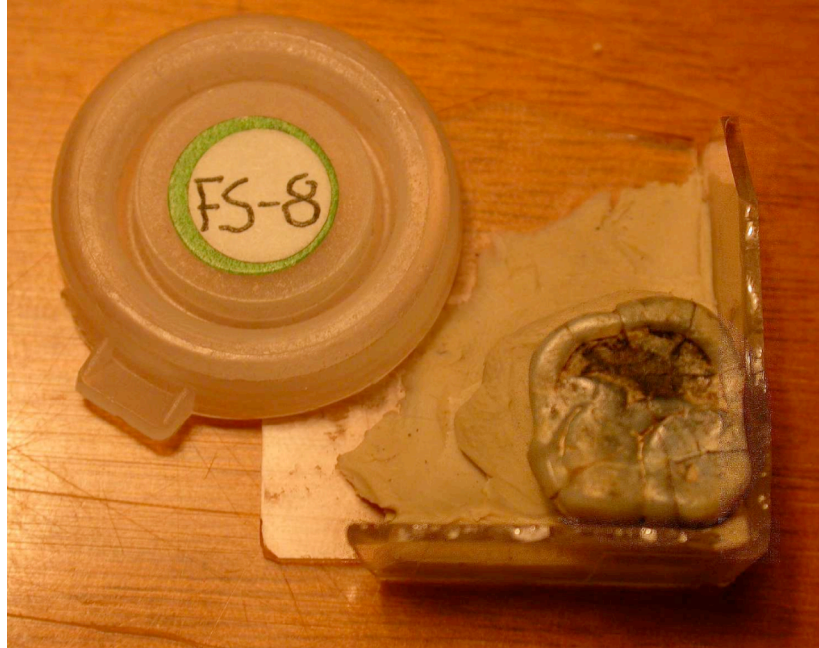
Figure 7.3. Customized specimen platform with tooth fixed in viewing position.
