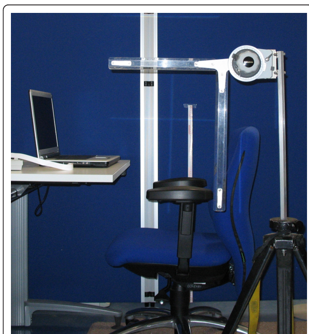
Figure 2 Study set-up. The workstation with adjustable ergonomic chair and desk as well as the adaptable protractor are displayed.
