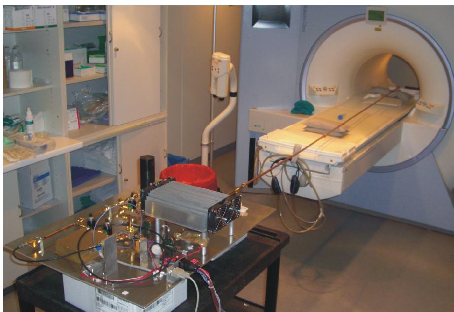
Figure 4.3: The principle setup of the DNP system in the MRI scanner: The DNP polarizer is placed inside the bore of the imaging magnet, right next to the imaging object, represented by a mouse. The microwave source is placed well outside the bore, keeping it out of the large stray field. Power transmission is accomplished via a 3 m piece of waveguide.
