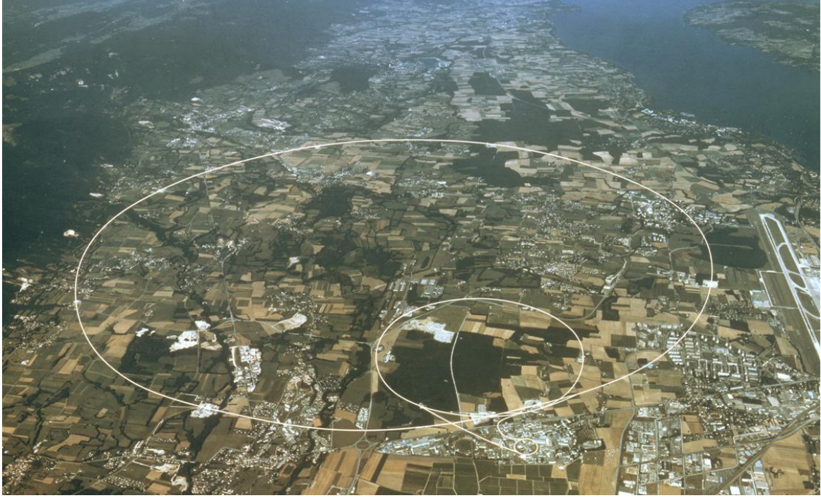
Figure 3.1: Aerial view of the CERN accelerator complex and the surrounding region of France and Switzerland; The LHC (large ring) and the SPS (smaller ring) cross each other close to the CERN main site. Following the LHC to the left, a bright spot on the LHC marks the ALICE experimental area [123].
