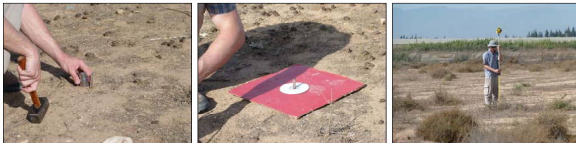
Figure 4. Ground control point (GCP) installation workflow (Photo: W. d'Oleire-Oltmanns 2011).
