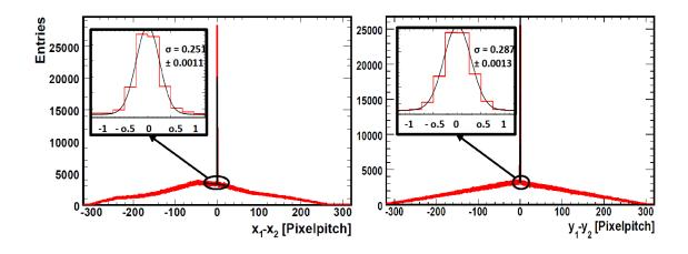
**Figure 3:** Position residual plot of the two demonstrator stations in x- (left) and y- (right) coordinate with a pixel pitch of 30  $\mu$ m. The zoomed insert shows details of the position correlation, together with a gauss fit.
