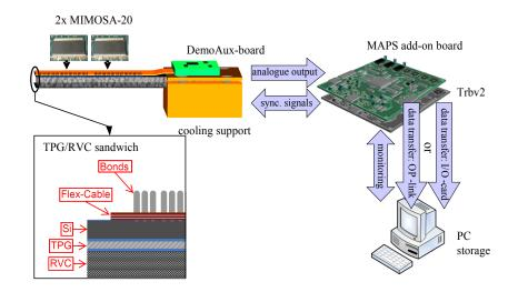
Figure 1: Sketch of MVD-demonstrator setup: Demonstrator module and R/O, DAQ.
