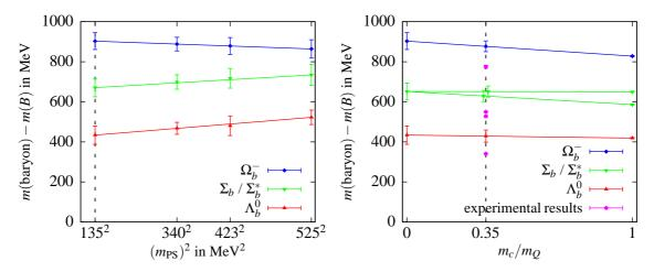
**Figure 2:** left: linear extrapolation of static-light mass differences in  $(m_{PS})^2$  to the physical u/d quark mass corresponding to  $m_{PS} = 135 \,\mathrm{MeV}$ ; right: linear interpolation between lattice static-light and corresponding experimental charm-light mass differences in  $m_c/m_Q$  to the physical b quark mass corresponding to  $m_c/m_b = 0.35$ .
