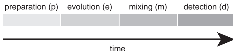
Figure 4.7: General pulse scheme of any 2D-NMR experiment.
