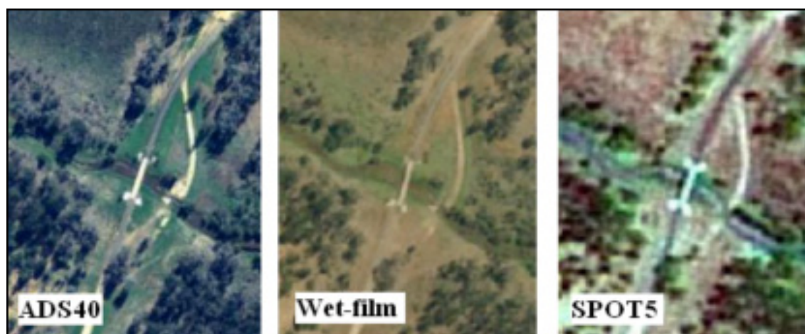
Fig. 2. Visual differences between ADS40, wet-film aerial photography and SPOT5 imagery (Black & Peasley 2008).
