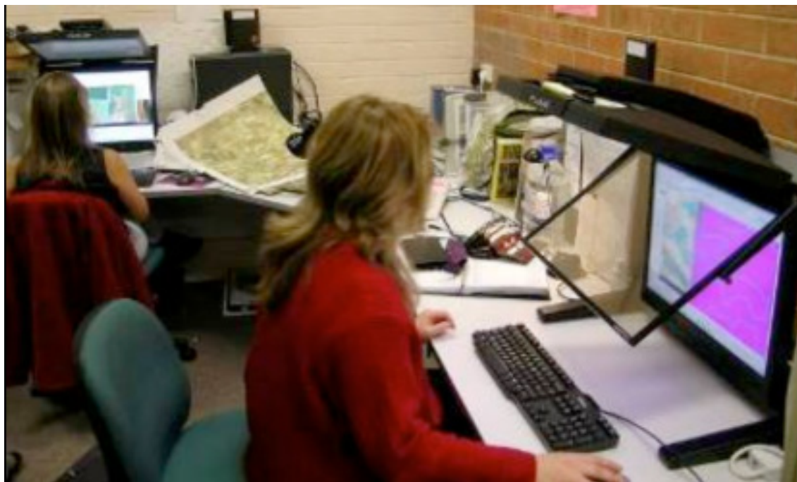
Fig. 3. DAPI operators at 3-D Planar workstations using Stereo Analyst for ArcGIS map software.
