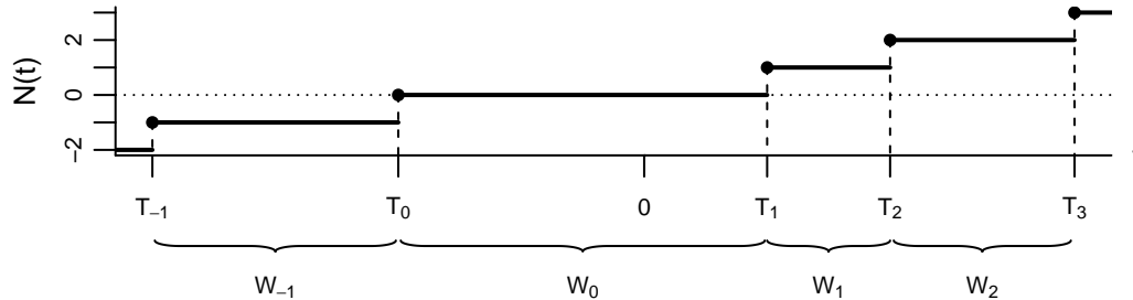
Figure 1.4: Point process on the real line with illustration of the relationship between the nondecreasing inter-valued step function N(t) , the sequence of time points \{T_i\} and the sequence of intervals \{W_i\} .
